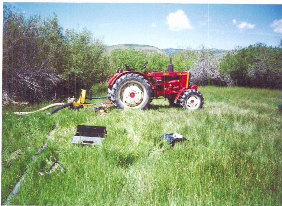
Plate 1 - Belarus diesel tractor with PTO drive.
