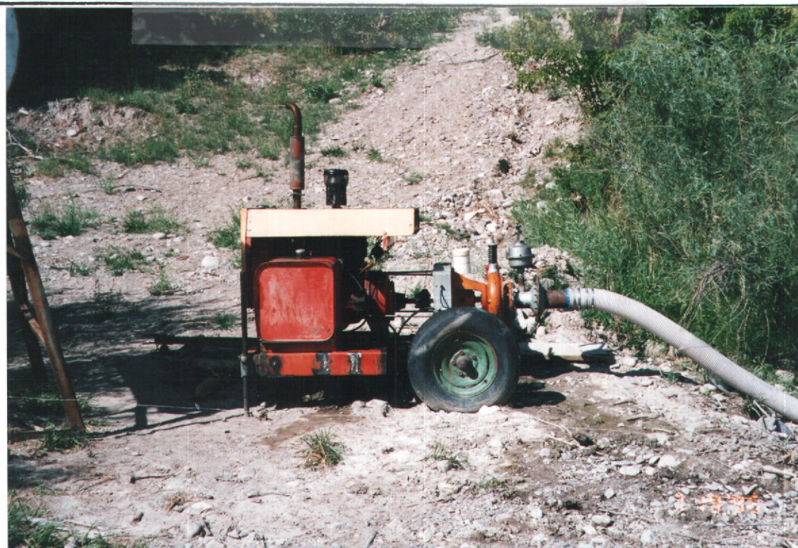
VIEW OF PORTABLE PUMP SYSTEM
