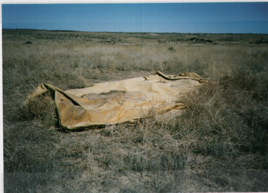
Fig. 2 - Portable 10,000 gallon storage tank.
