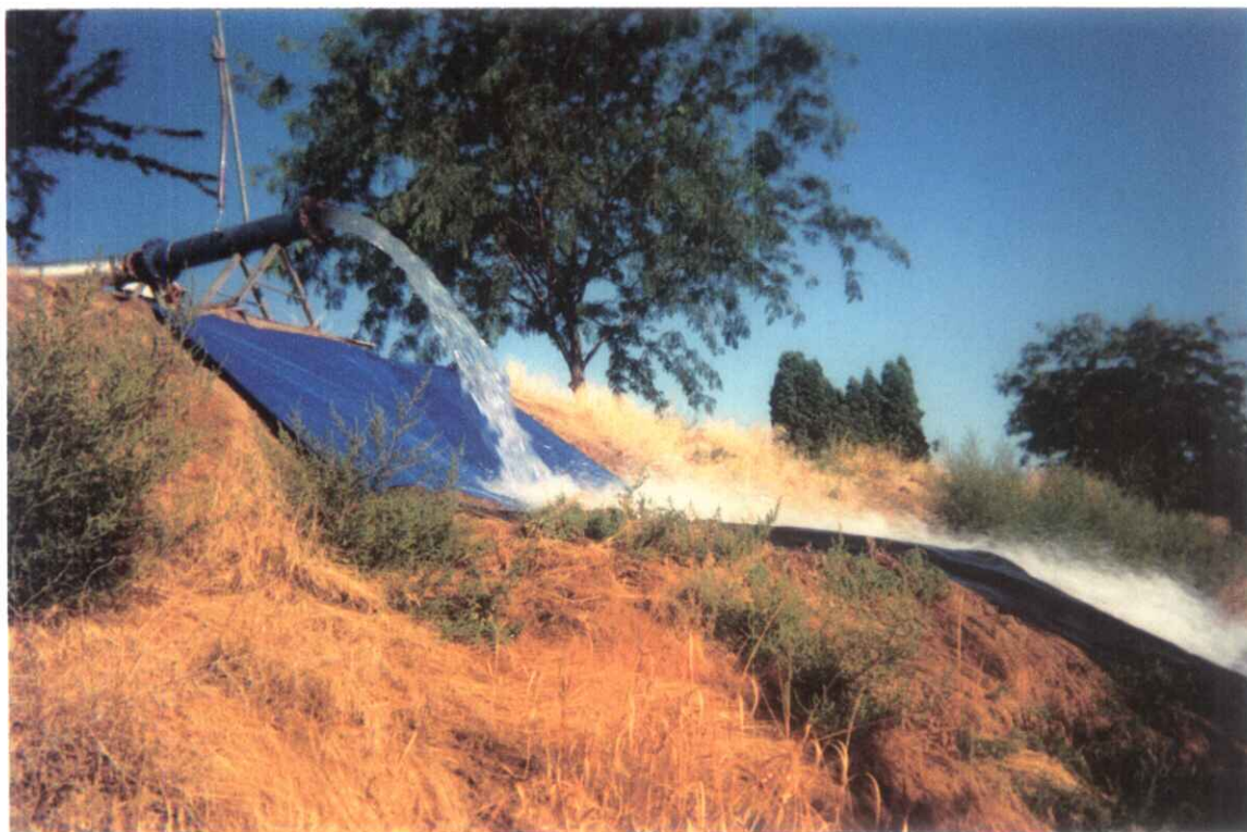
Figure 13. Photographs of the circular orifice weir discharge during hydraulic testing of the Caldwell municipal supply Well #4-B. The well was discharged at rates between 1,000 gpm and 1,710 gpm for the stepped discharge testing and a constant discharge test was conducted for 8½ hours at 1,250 gpm. Discharge was to the basalt rim rock of Canyon Hill above Mason Creek.
