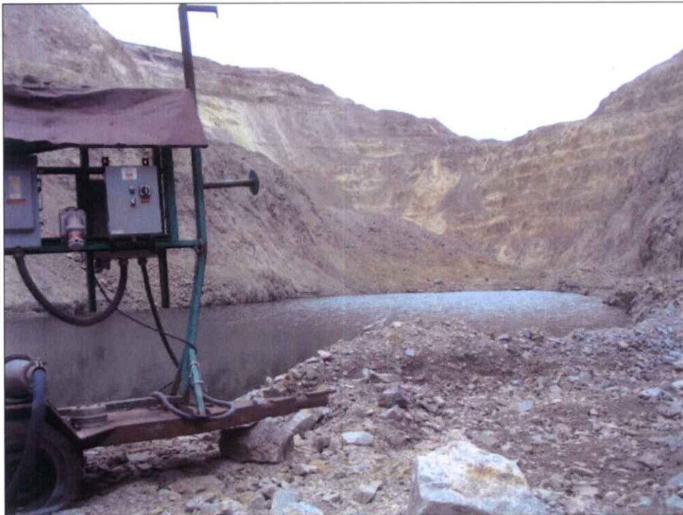
Photo 2: Intermediate level mine pit sump. Water from the lower elevation pit (in the background) is diverted to this pond.
