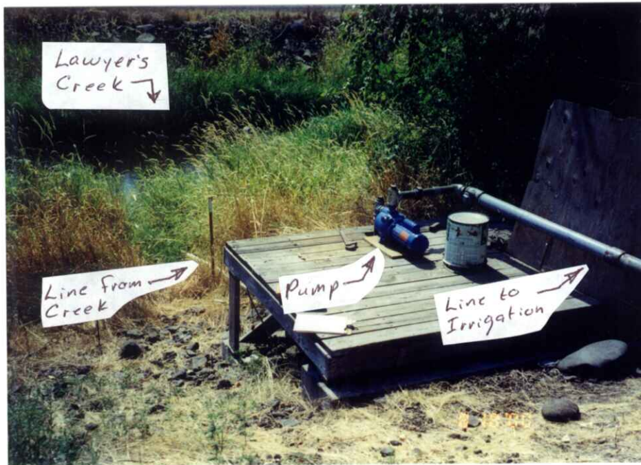
Photo 1. Showing Point of Diversion (POD).
