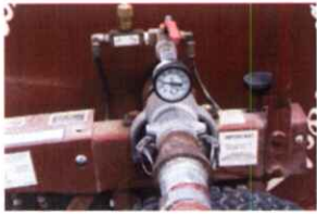
38 PSI Machine Inlet Pressure indicated.jpg
