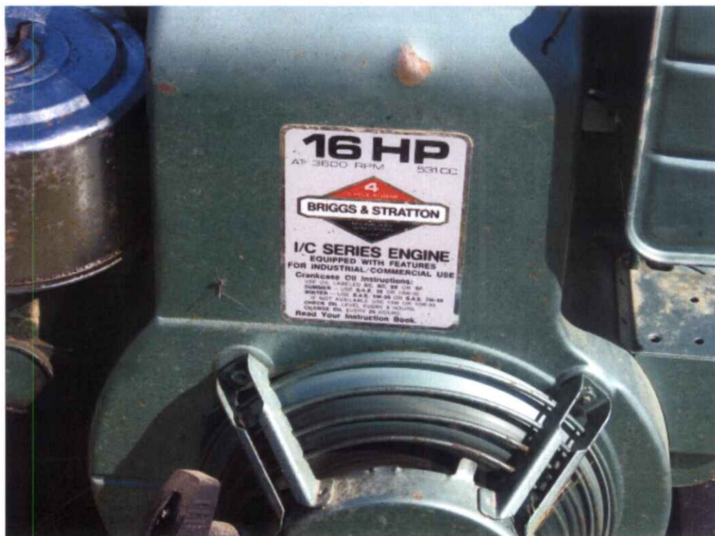
95-9060 16 HP Pump data plate on mobile dolly
