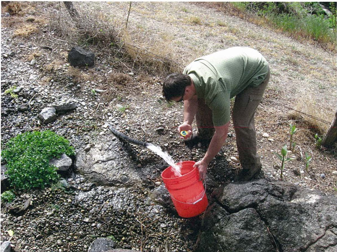
FIGURE 9: Measuring system capacity at “freeze line” discharge point
