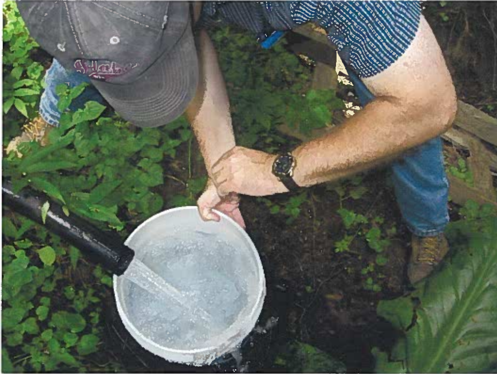
95-8998 JUL 08 Eight GPM at Bypass
