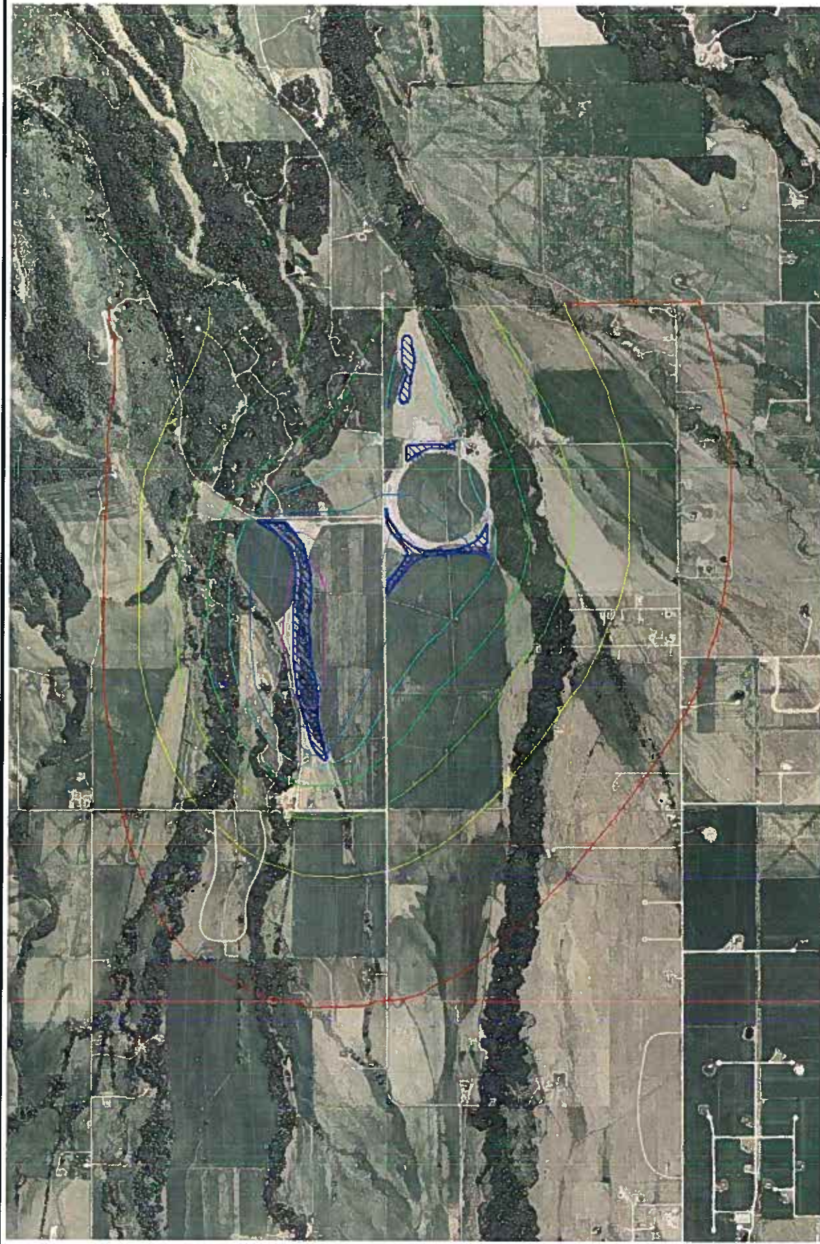
FIGURE 4: AQUIFER MOUND CREATED BY RECHARGE MODFLOW GROUNDWATER MODEL TETON RANCH AQUIFER
