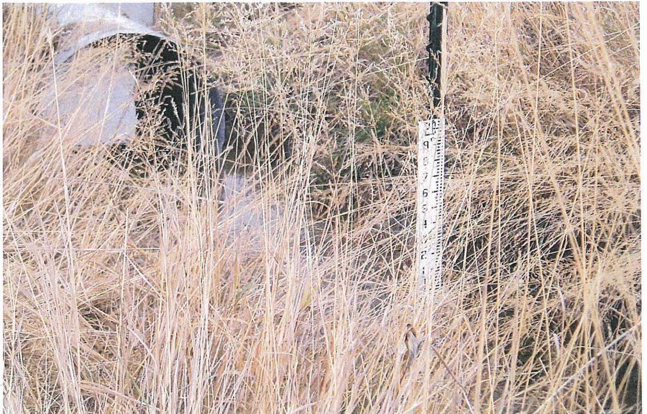
Staff gauge purchased at IDWR in Idaho Falls installed in Fall of 2009.
