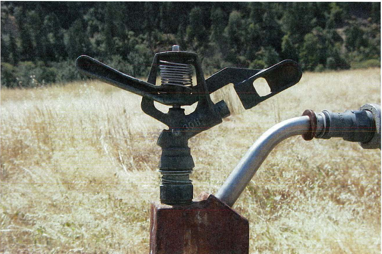
Figure 6: Typical sprinkler head installed on wheel line, Rainbird 30H.
