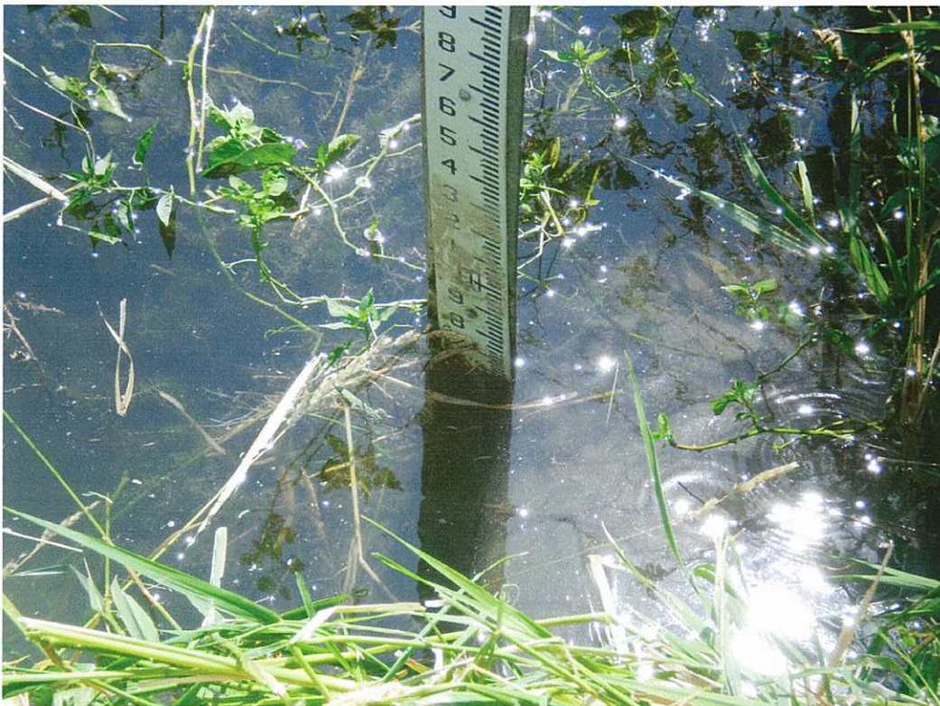
Staff gauge downstream of concrete pipe culvert
