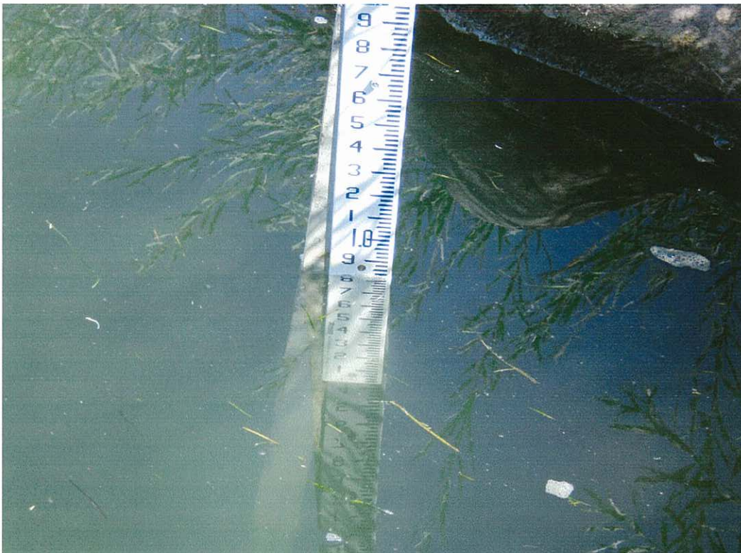
Staff gauge on river side
