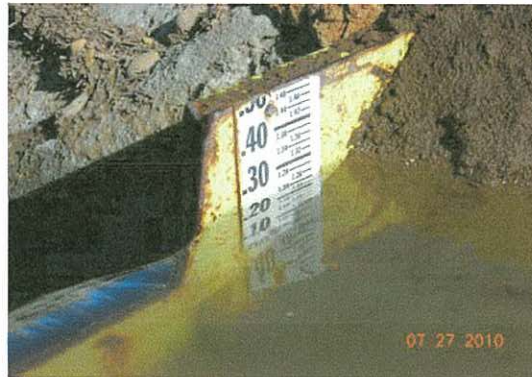
24-inch Cipolletti Weir reading 0.245 inches = 0.817 cfs (367 gpm) Ground water only, no surface water at time of measurement
