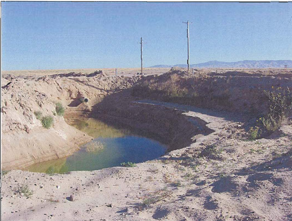
Photo 4: Well water is delivered to this pit where it is subsequently rediverted for gravel washing.
