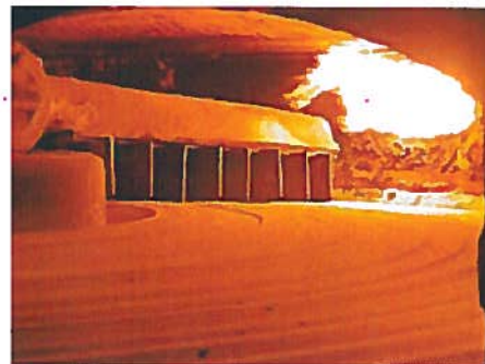
Interior of a roasting furnace (Courtesy of Molymet, Chile)
