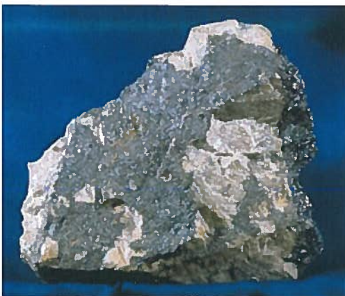
Molybdenum ore; dark gray areas are \text{MoS}_2 , while light areas are worthless rock called gangue
