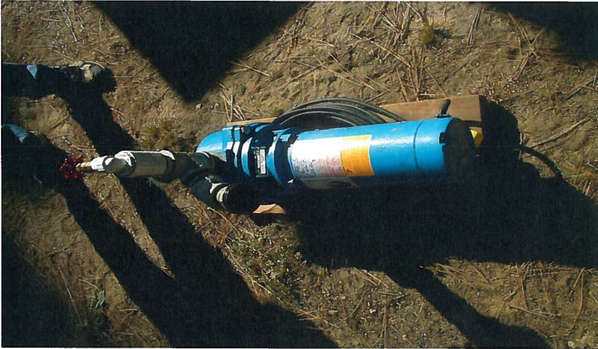
1.5 hp pump (in garage for winter) used to divert water from South Fork Payette River
