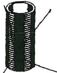
TYPICAL LINESHAFT BEARING C93200 BRONZE
