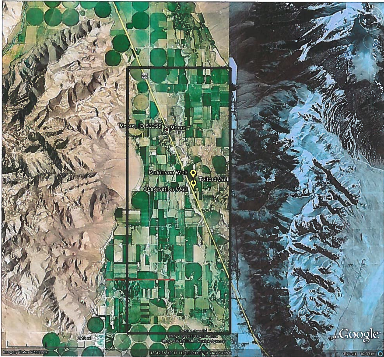
Figure 4-1 Outline of the boundaries used in the AQTESOLV forward solution calculation. Note for scale that the red line is 10,000 ft long.
