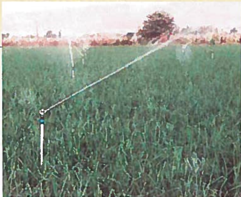
Solid Set. Aluminum pipe, PVC, or Polyethylene.
