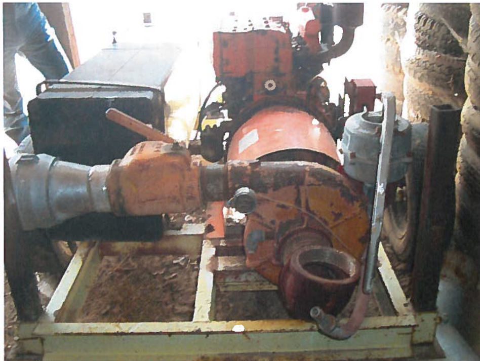
61-7600 Exam 5/30/2012: Diesel motor and pump on trailer (portable) for irrigation system.
