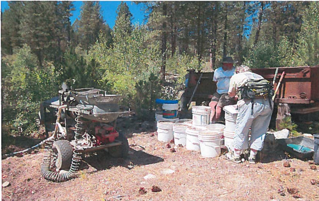
Another view of processing plant. Dump truck bed also used to wash tailings.
