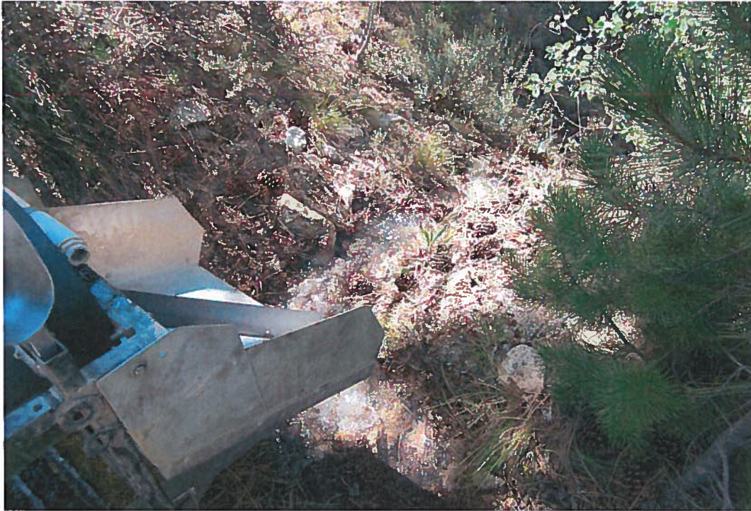
Water flows from trommel to settling pond.
