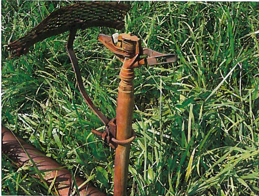
Photo looking southerly at 2" above ground pipes for the handlines.
