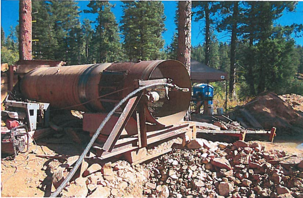
Trommel made by Clarence McReynolds. Water is pumped from Fall Creek to the trommel.
