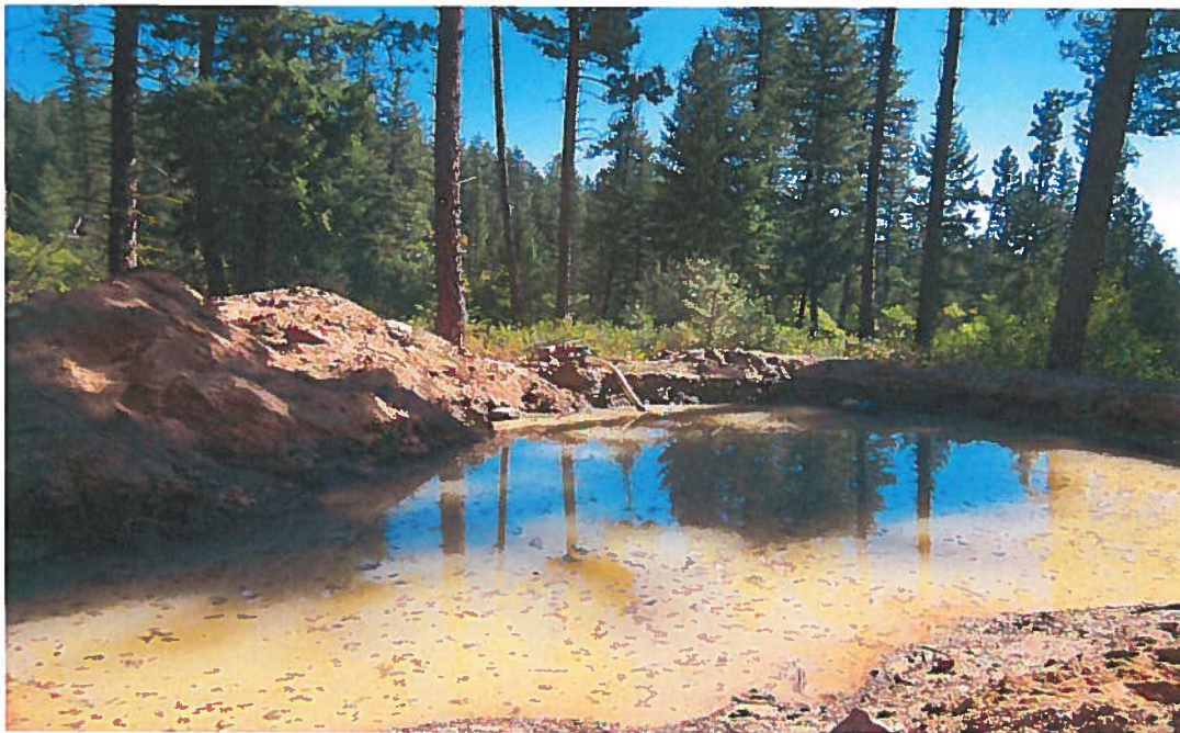
Water flows from the trommel into this settling pond. The pump seen far side is the recycling pump.
