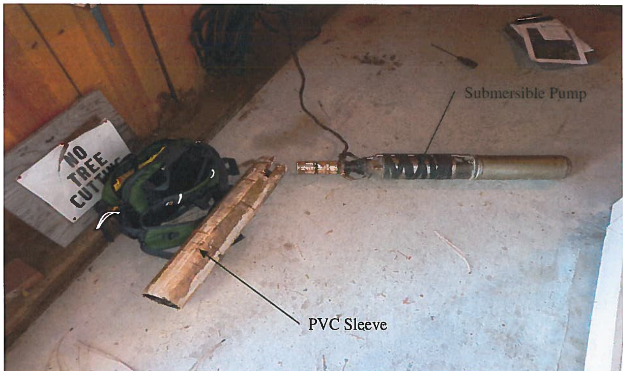
View of the submersible pump and PVC sleeve in which pump is inserted prior to installation in the diversion ditch.
