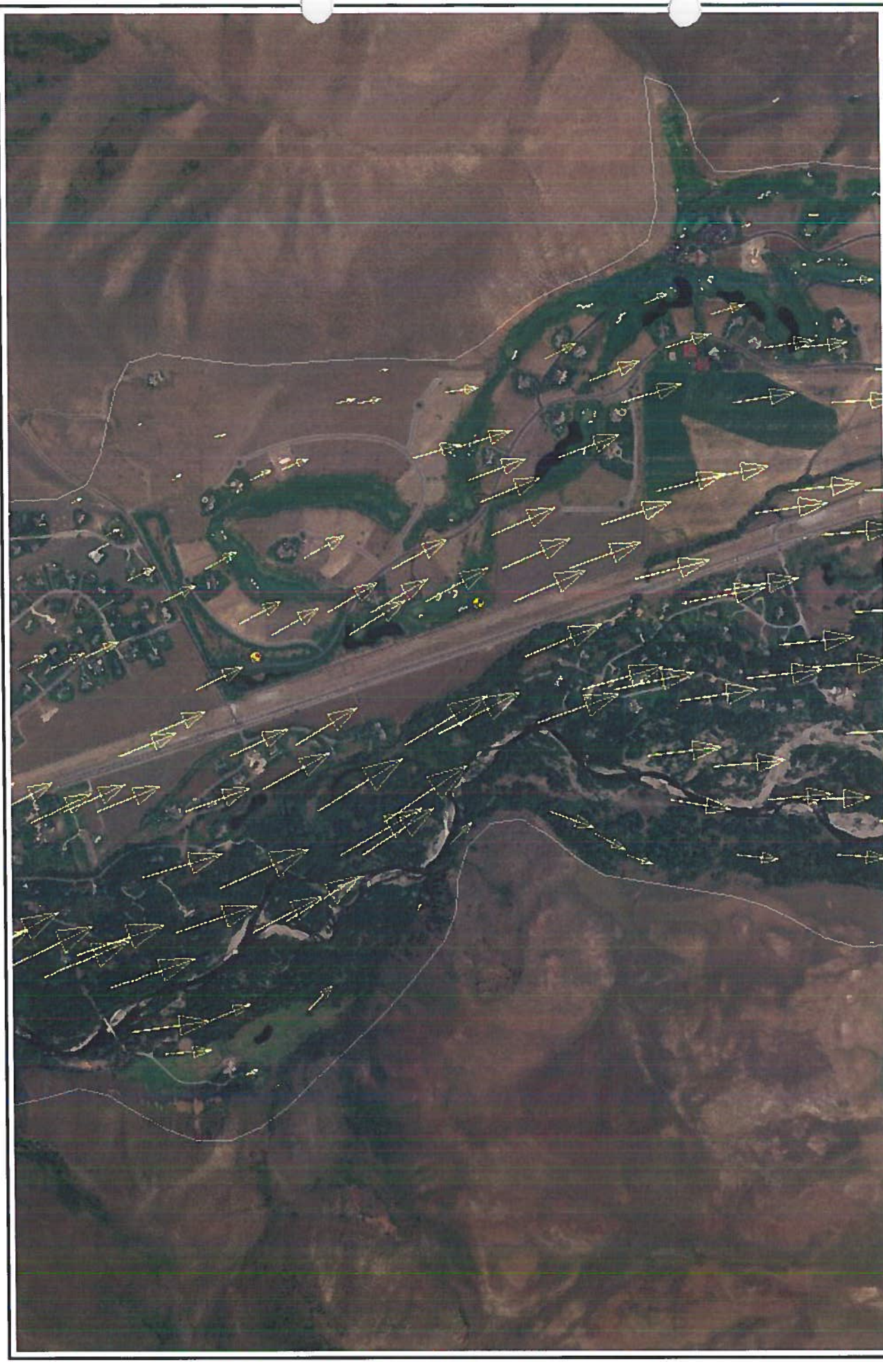
FIGURE 11: BIG WOOD AQUIFER FLOW VECTORS NEAR VALLEY CLUB, INC PROPOSED RECHARGE PROJECT LARGER FLOW VECTORS INDICATE HIGHER VELOCITIES CONCENTRATED NEAR THE BIG WOOD RIVER
