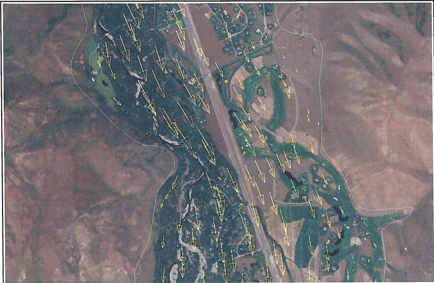
FIGURE 11: BIG WOOD AQUIFER FLOW VECTORS NEAR VALLEY CLUB, INC PROPOSED RECHARGE PROJECT
