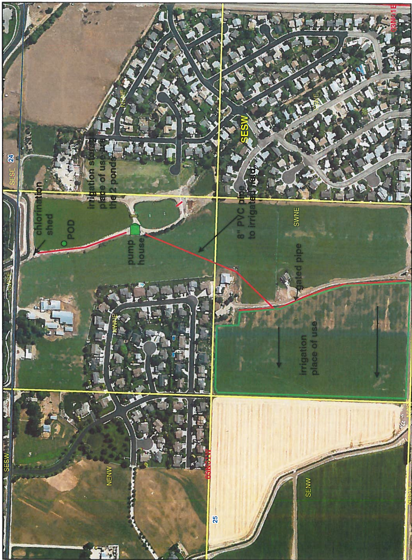
63-12251 -- 2013 NAIP PHOTOGRAPHY. Diagram of places of use, storage, treatment and diversion of water from the waste ponds to irrigated field to the southwest.
