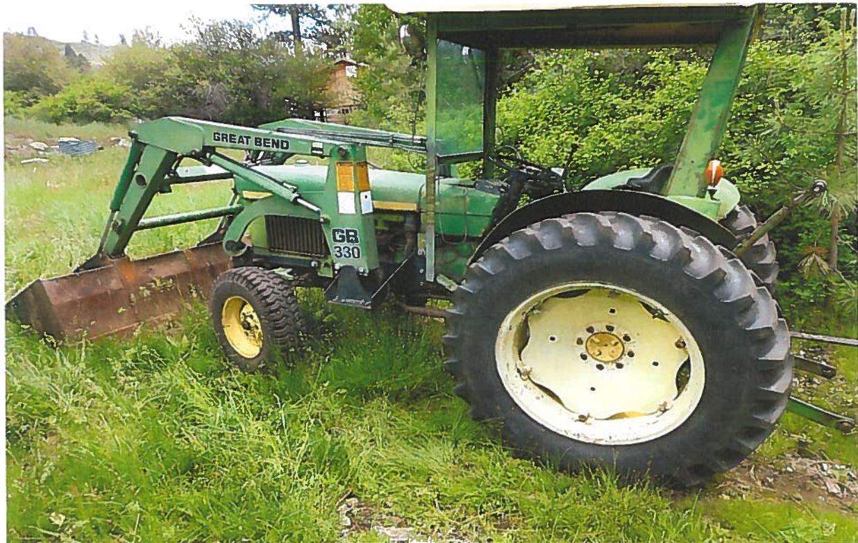
View easterly of the tractor which provides the motor power to operate the pump.
