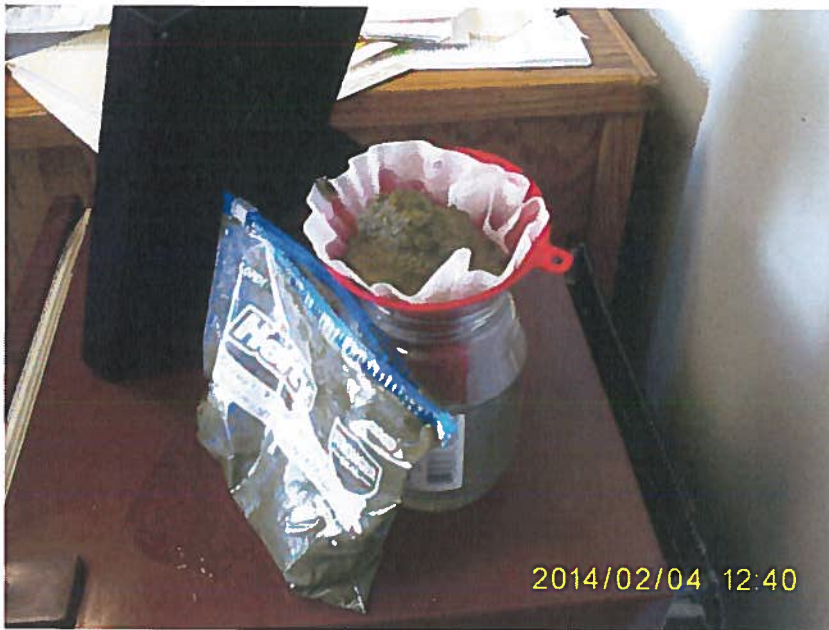
Photo 7792. Warm Springs sediment sample draining in a coffee filter.
