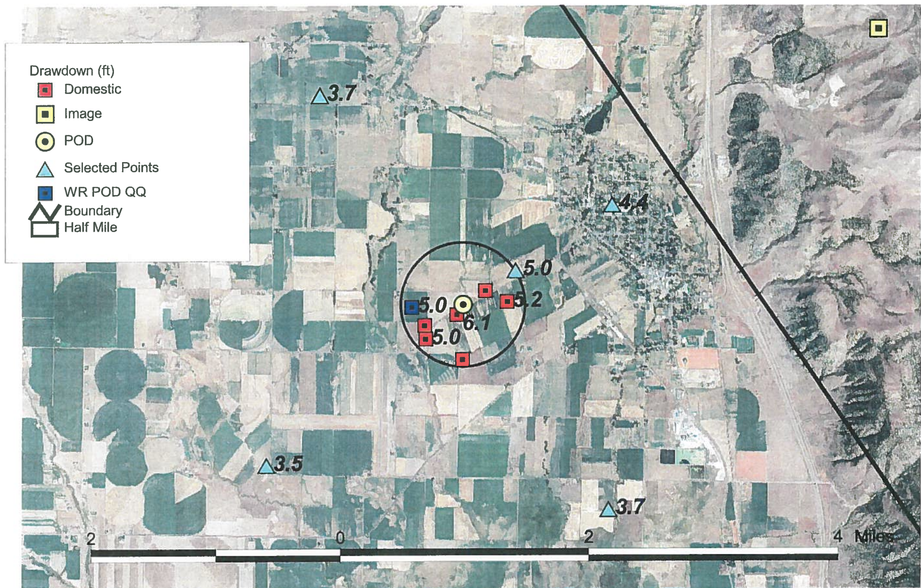
Figure 3 - Theis Drawdown Calculations Hartvigsen WR Permit Application Project 14-0048
