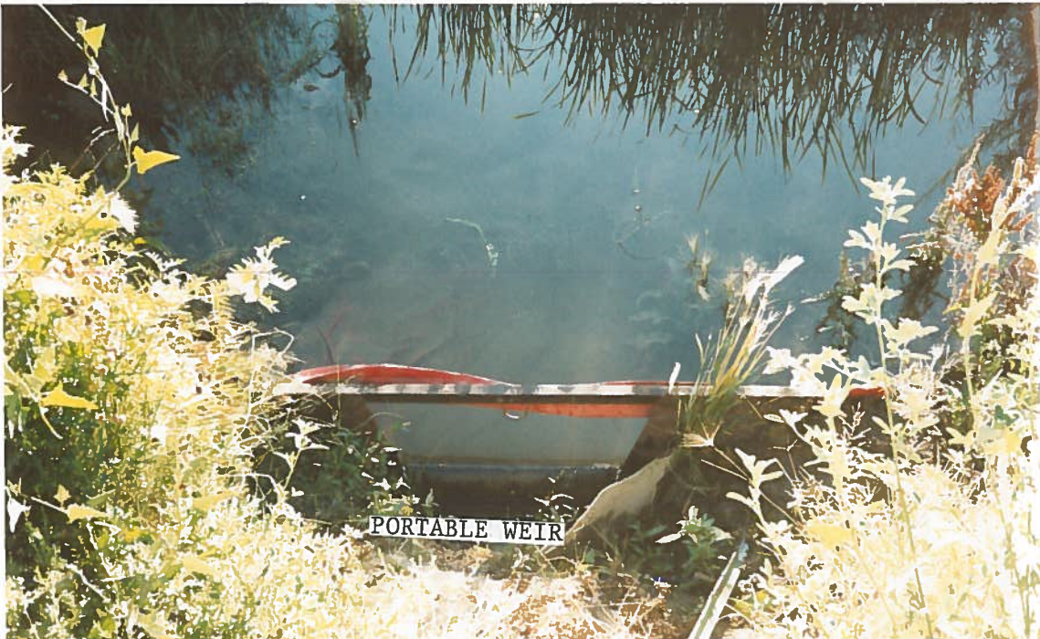
PHOTO FOUR- Taken looking east shows the stilling pool and portable weir installed for the purpose of doing a water measurement of the spring flow.
