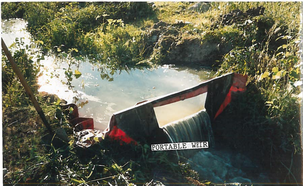
PHOTO SIX- Taken looking southeast at a portable weir installed for the purpose of doing a water measurement of the spring flow.
