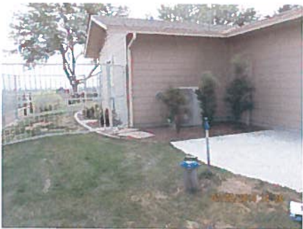
The old domestic well (left) has been retrofitted to operate as an injection well, with a heat exchanger (right) inside the home. This system cools and heats the home on a seasonal basis.
