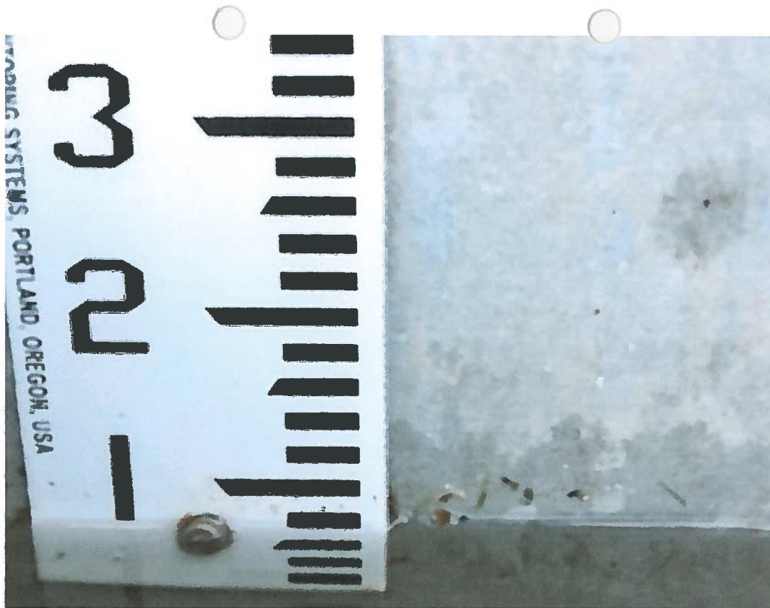
Staff gauge on weir showing H = 0.07 feet.
