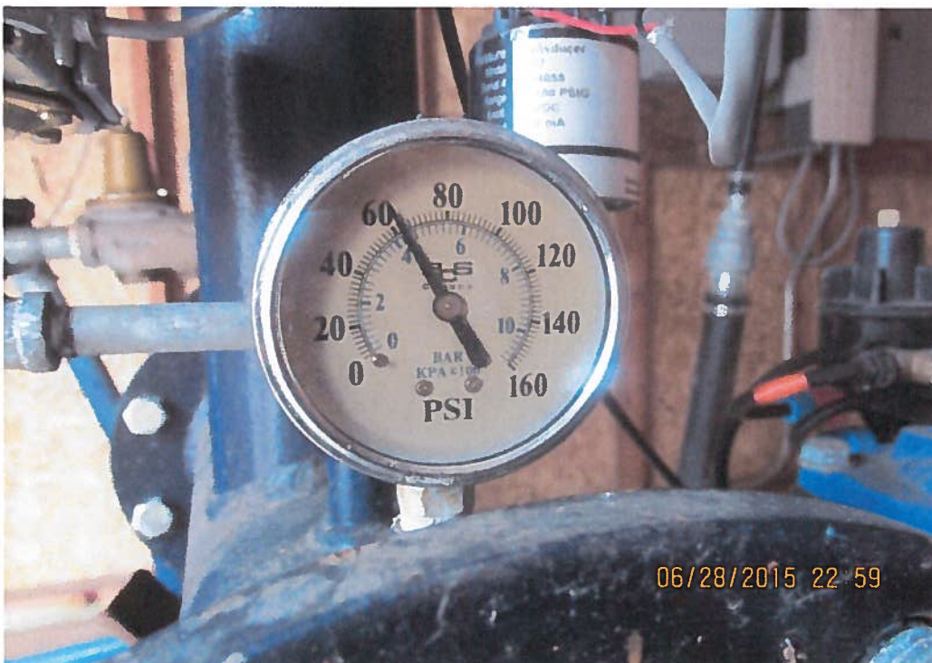
Pressure gauge reading 60 PSI
