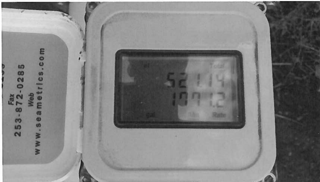
Photo 5: Photo of the Seametrics readout screen. The Seametrics permanent flowmeter averaged 1,768 gpm over a 9 minute 13 second time period while the 10-minute averaged portable flow meter measurement computed to 1,713 gpm, a difference of slightly more than 3%.
