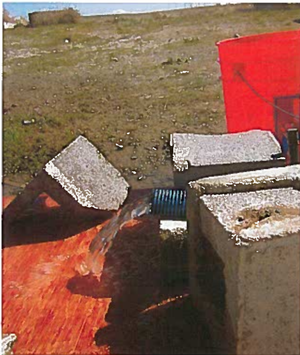
13 gpm discharge and top of 1.25-inch sounding tube with measurement point identified
