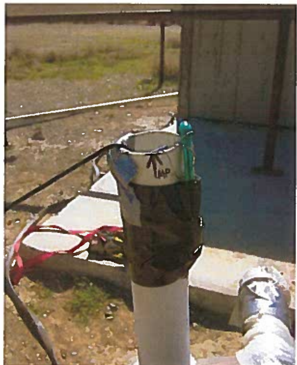
13 gpm discharge and top of 1.25-inch sounding tube with measurement point identified
