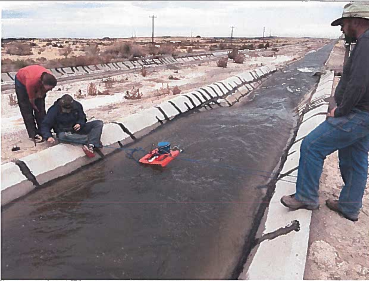
Dennis Owsley using Acoustic Doppler Current Profiler to measure water passing through Basin & Land ditch.
