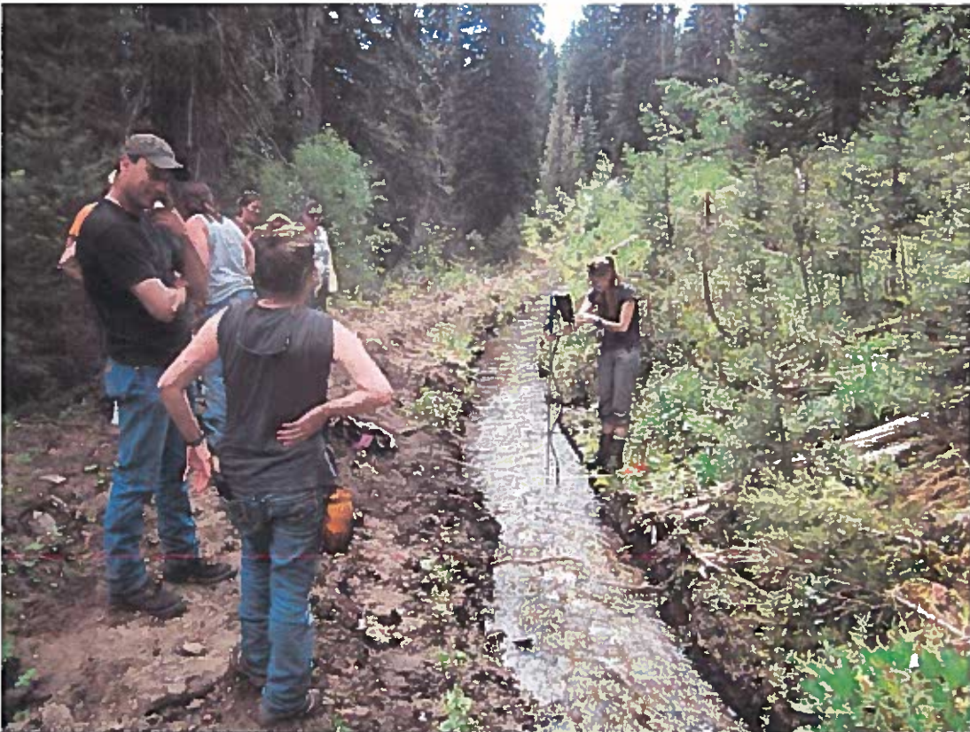
6. Looking downstream on connection ditch. Location of flow measurement (approximately 1.0 cfs. See attached "Ditch 1" flow meter data)
