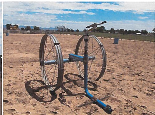
Spray King Sprinkler used for dust abatement for corral
