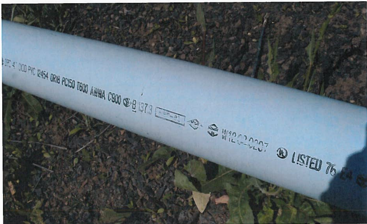
Pipe scrap. 4-inch C900 PVC
