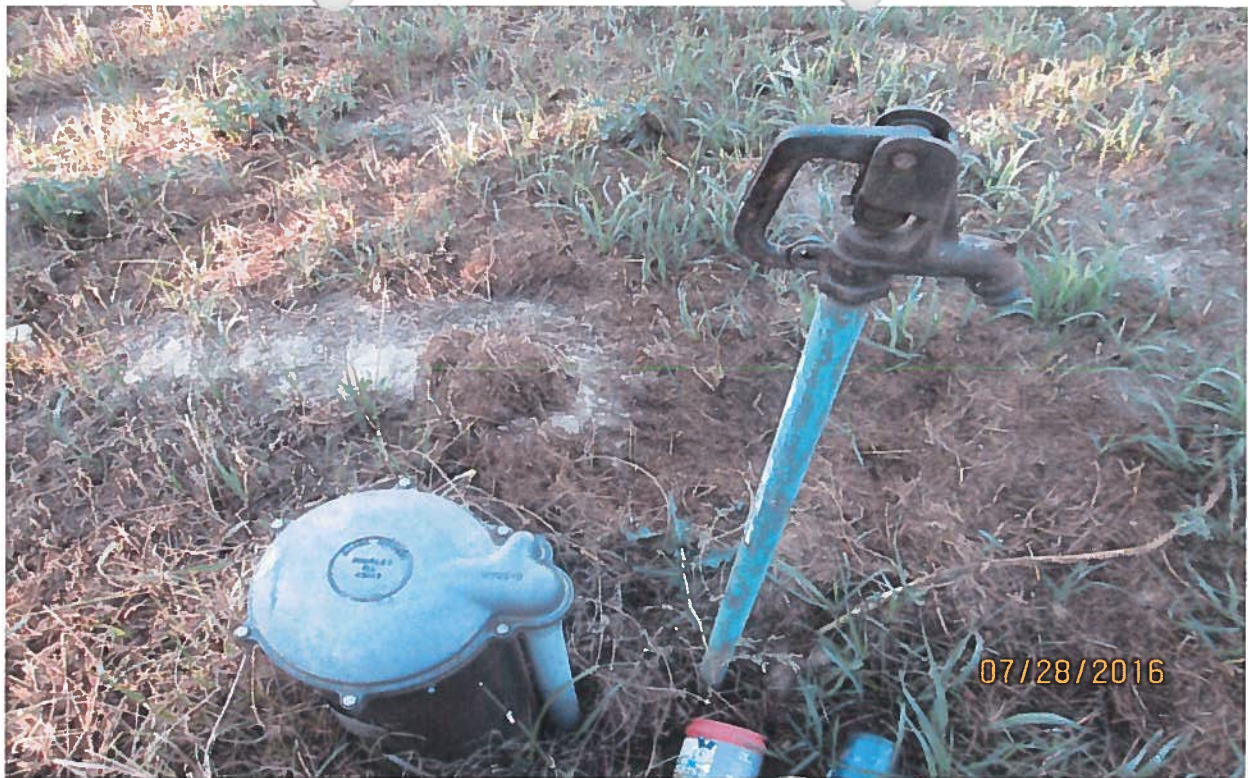
Well and frost free used for 5 gallon bucket test. 5 gallons in 12 seconds is equal to 25 gpm or 0.06 cfs
