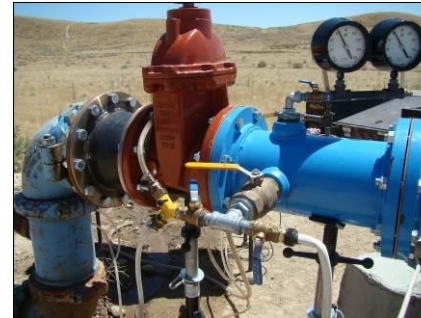
7-17-2016 – Flow-meter registering ~2,125 gallons/minute during second day of 4-day (96-hour) long aquifer test of Spring Valley Municipal Well #2. At end of the test, totalized flow matched the instantaneous readings and pumping time.
