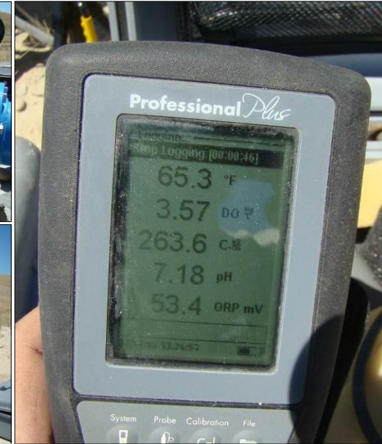
7-17-2016 – HLI sampling equipment being used for field-measured water chemistry parameters for IDEQ “New Source Monitoring” of SV Well #2 discharge water during 2,125 gallons/minute aquifer test.
