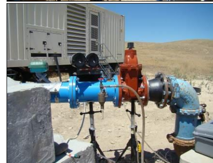
7-17-2016 – HLI sampling equipment being used for field-measured water chemistry parameters for IDEQ “New Source Monitoring” of SV Well #2 discharge water during 2,125 gallons/minute aquifer test.
