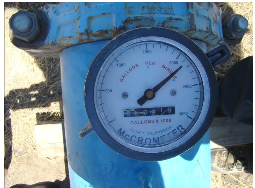
7-17-2016 – Flow-meter registering ~2,125 gallons/minute during second day of 4-day (96-hour) long aquifer test of Spring Valley Municipal Well #2. At end of the test, totalized flow matched the instantaneous readings and pumping time.
