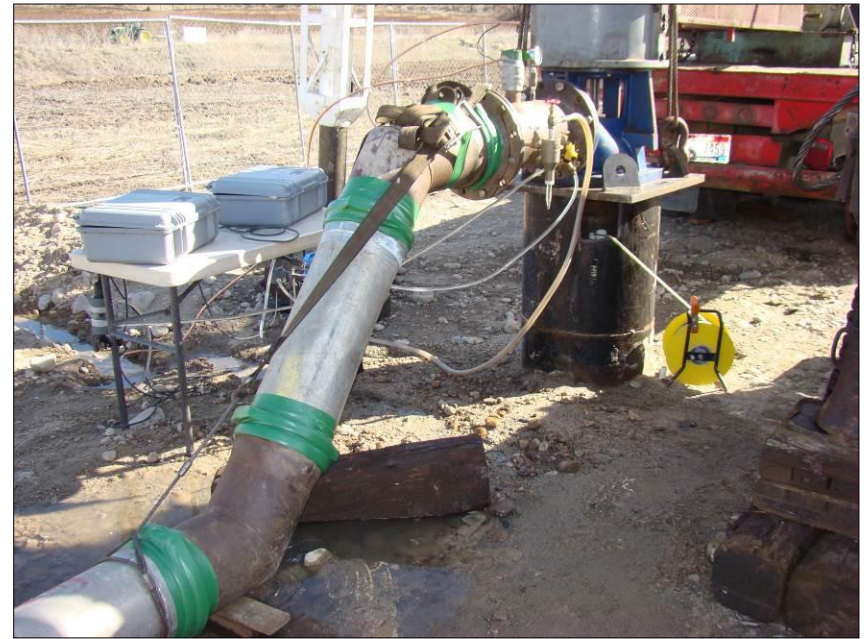
2-24-2016 – HLI sampling equipment being used for field-measured water chemistry parameters for IDEQ “New Source Monitoring” of SV Well #1 discharge water during 2,700 gallons/minute aquifer test.
