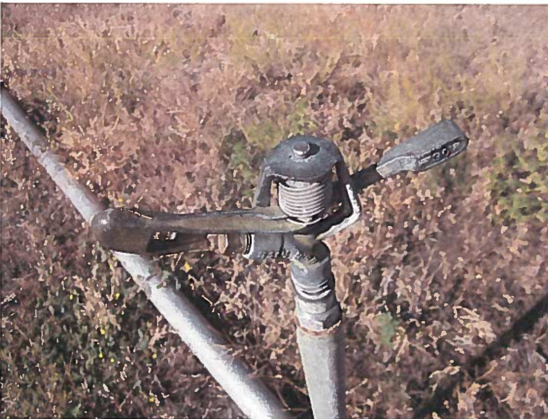
8. Sample sprinkler head. 30WS, 1/8 inch nozzle sprinkler heads. 4 lines run at one time with one sprinkler head every 40 feet.
