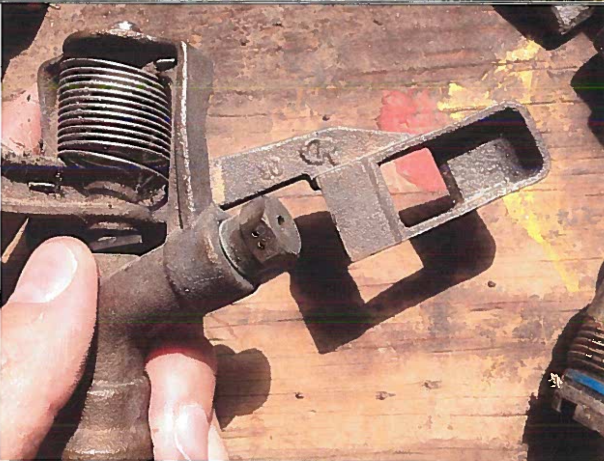
All sprinklers are fitted with 9/64" nozzles.
