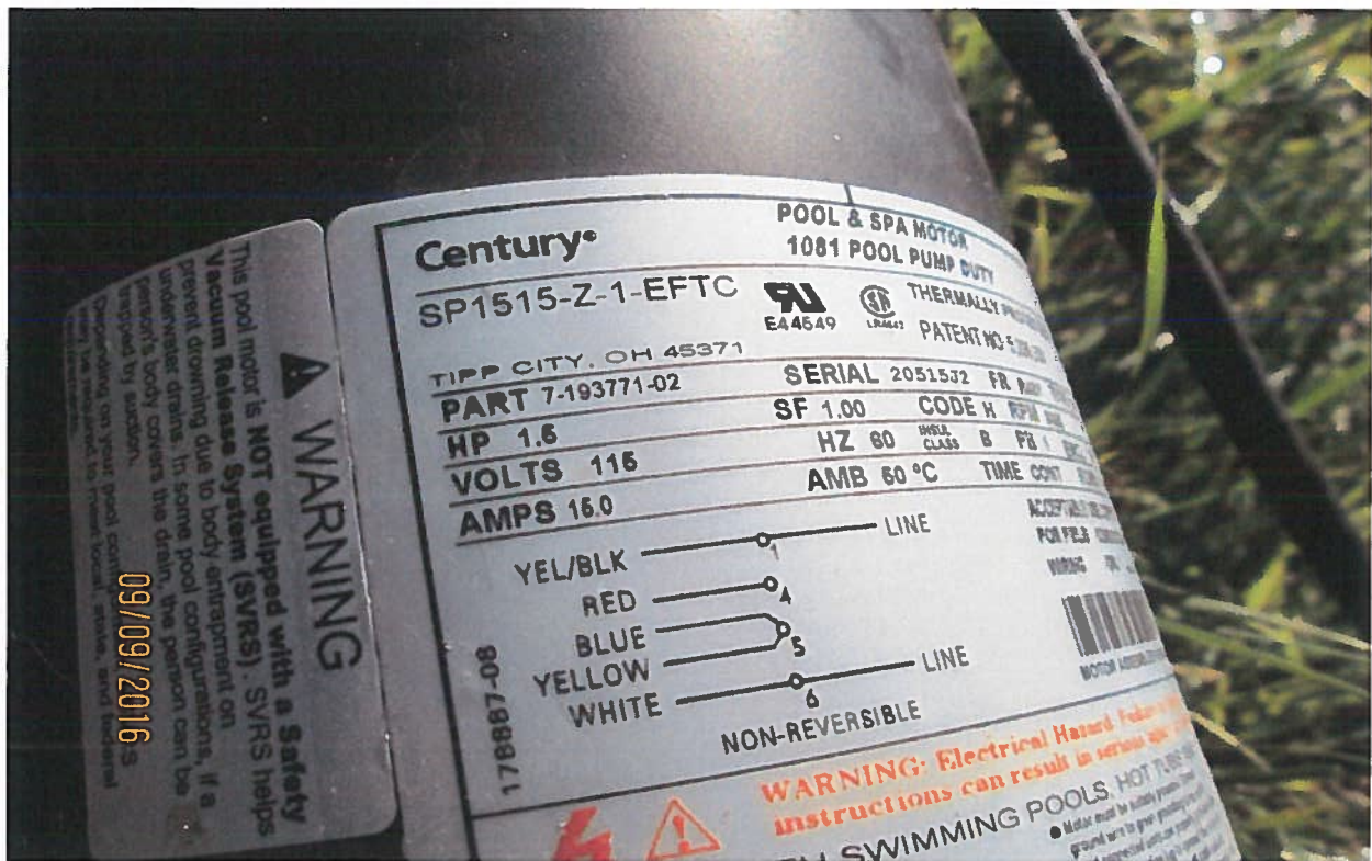
1.5hp pump used for irrigation from storage tank.
