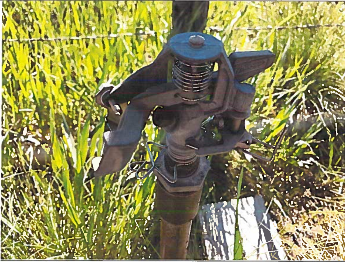
Sprinkler using 1/8" nozzle.
