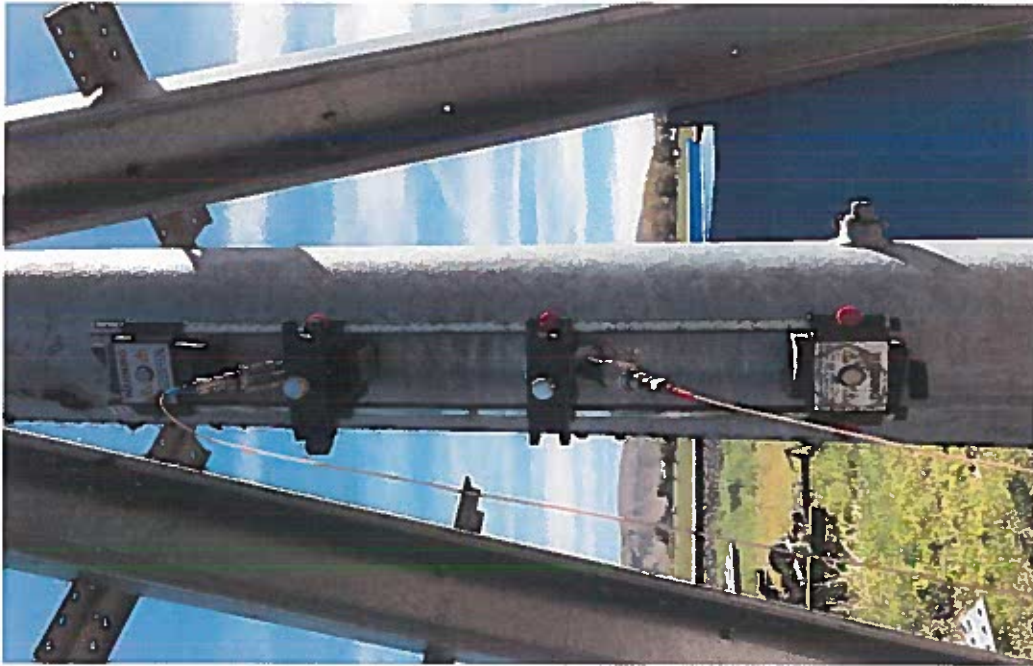
Picture of GE Panametrics measurement system in use near pivot head.
